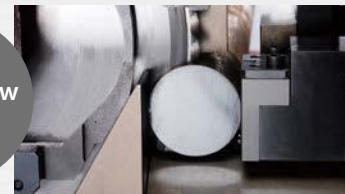
Metal is cut by a circular band-shaped blade
