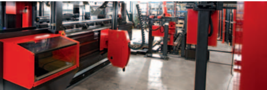
An automatic storage system (very top in background) is used for the provisioning of the production units.
